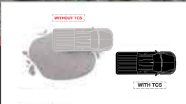
TRACTION CONTROL SYSTEM (TCS)
